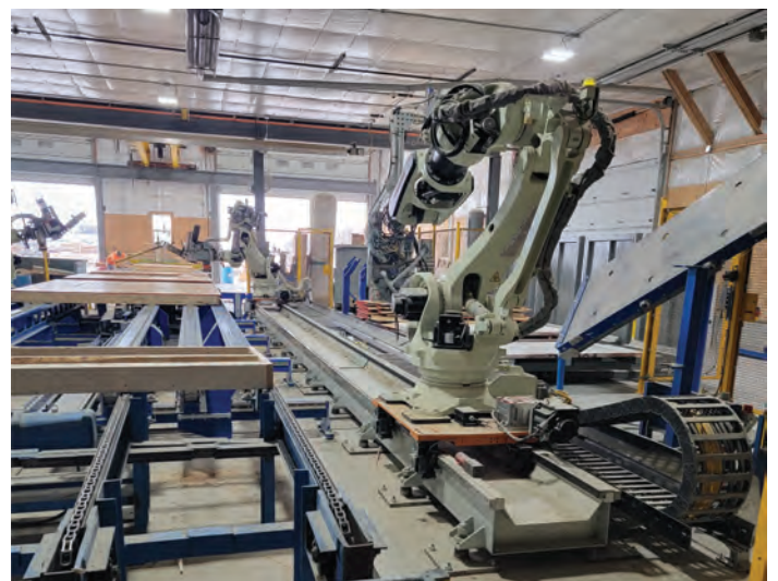
The Kawasaki BX250L robot can lift 250 kg, and offers a through-arm cable design for added convenience.
