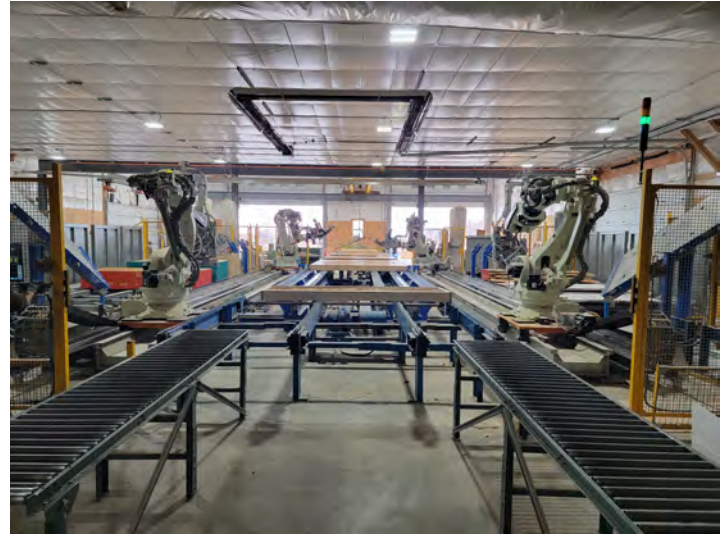
Kawasaki robots are used to mount cumbersome OSB sheathing to pre-framed walls and cut out windows and doors.
